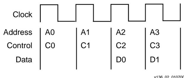
**Figure 2: Bus Operations for Pipelined ZBT SRAM**
